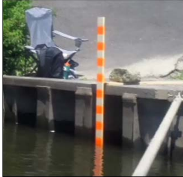
Figure 4: Visual Wake Measurement near a Bulkhead
